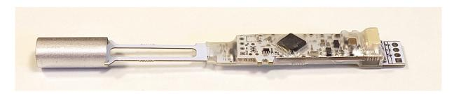
SKS21 is a temperature and relative humidity sensor module with very fast response time, designed for UAVs and miniature radiosondes. Special care has been taken to minimize the self-heating even in low air pressure.
