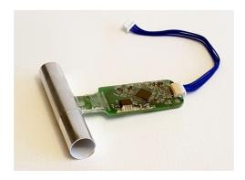
SKS2 is a temperature and relative humidity sensor with very fast response time, designed for UAVs. The sensor elements are protected by a reflective tube that is oriented in the direction of the wind flow.
