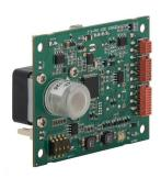
High-resolution ozone measurements for Sparvio, with built-in fan.
