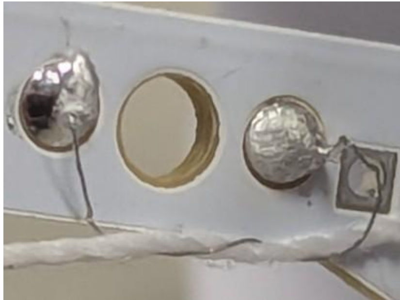
The tightened tether line is twisted around the metal wire.
